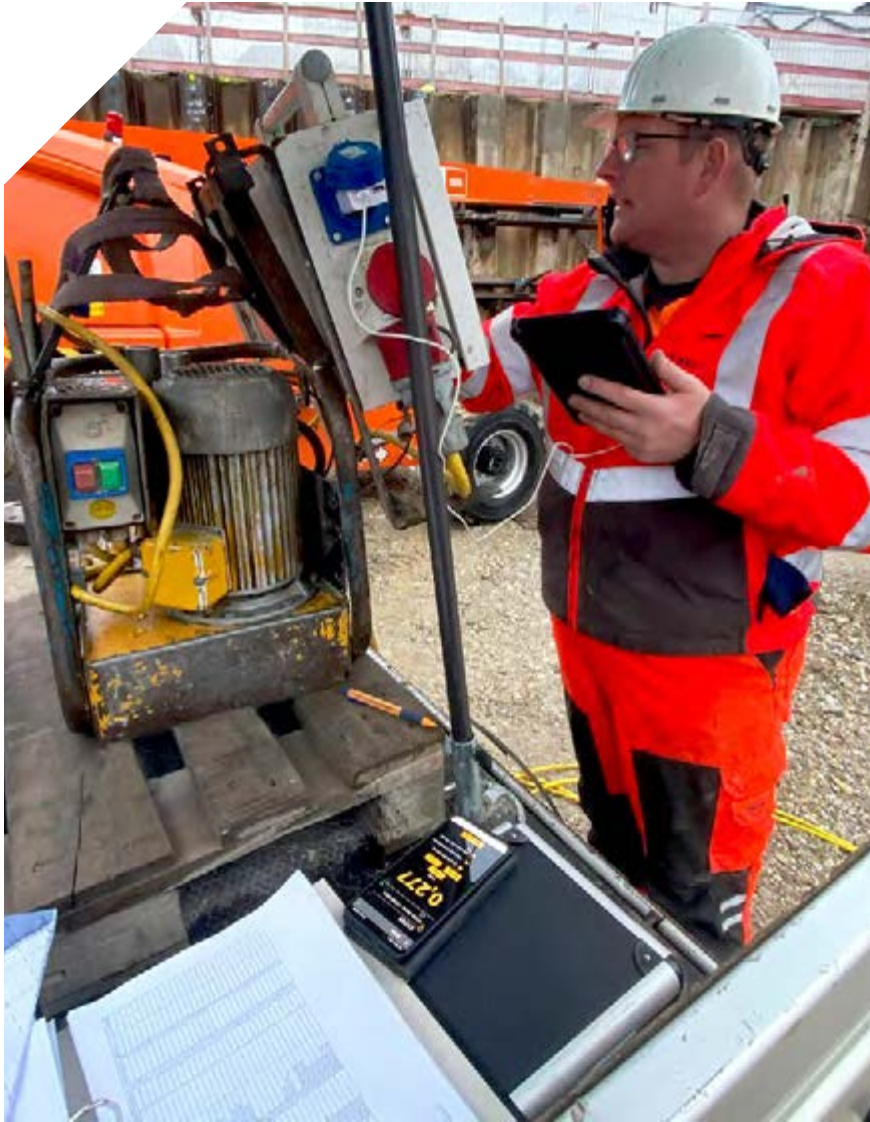
GAUGE WITH BLUETOOTH transmission to the anchor stressing app
