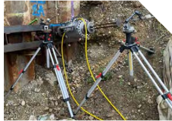
GAUGE WITH BLUETOOTH transmission to the anchor stressing app
